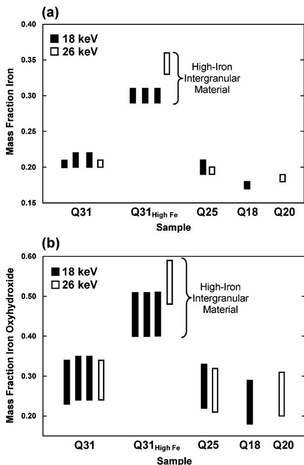
**FIGURE 4.** Approximated mass fraction iron (a) and mass fraction iron oxyhydroxide (b) in the intergranular material for different soil samples and multiple measurements of the same sample. Some measurements were made at 18 keV and others at 26 keV. Ranges in values represent uncertainty in the possible iron oxyhydroxide and clay composition. Mass fraction clay is assumed to be 1 minus mass fraction iron oxyhydroxide.
