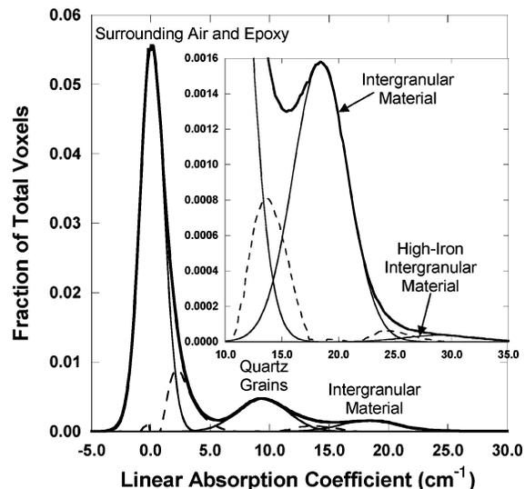
**FIGURE 3.** Histogram showing the fraction of voxels that are air or epoxy, quartz grains, and intergranular material for sample Q31. Inset is an enlargement of the intergranular portion of the histogram showing the high-iron intergranular region. Heavy solid line is the histogram of the data. Light solid lines are the best-fit Gaussian distribution. Dashed lines delineate voxels that overlap two regions (mixed-value voxels).
