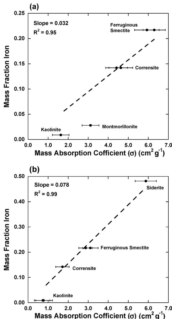
FIGURE 2. Regressions used to correlate measured  $\sigma$  with mass fraction iron for data collected at 18 keV (a) and 26 keV (b). Data were collected on mineral standards. Error bars represent  $\pm 1$  standard deviation of the measured  $\sigma$ . The regression lines were forced to intercept the origin.
