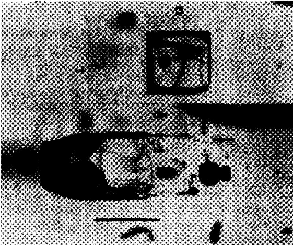
Figure 1. Photomicrograph of fluid inclusion in rock salt from Waste Isolation Pilot Plant, Carlsbad, New Mexico, before (upper) and after (lower) heating with an imposed thermal gradient of 1.5^{\circ}\text{C}/\text{cm} at 202^{\circ}\text{C} for 156 hours. The arrows denote the original boundary of the fluid inclusion. The scale bar represents a distance of 500\ \mu\text{m} . From Roedder and Belkin (1980).
