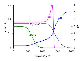
Figure 3. Concentrations of  $SO_4^{2-}$ ,  $Zn^{2+}$ , U(6) and pH from acid mine drainage along a flowline calculated with PHREEQC-2.
