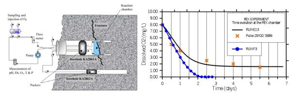
Figure 1. Setup of the REX in situ experiment (left) and time evolution of measured and computed dissolved oxygen (right). Computed values are shown for models considerin: DOC respiration (Run E13) and the combined effect of DOC respiration and methane oxidation (Run F3).
