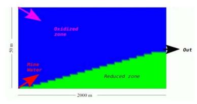
Figure 4. Outline of the model aquifer. The reduced zone contains pyrite.
