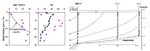
Figure 1. Regular flowlines in a phreatic aquifer (right) are contradicted by the age profile calculated from tritium/helium measurements in borehole DFG 1 (modified from Leuchs, 1988).
