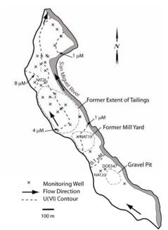
Figure 1. Naturita mill tailings site illustrating the monitoring wells, U(VI) concentrations, the extent of the former tailings piles and mill site, and the gravel
