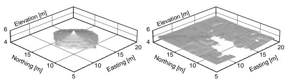
Figure 3: 1 g/L permangante iso-contour surface (left) and 1 percent DNAPL volume fraction iso-contour surface (right) at 14 days following initial permanganate injection. Injection point location was 12.5 m northing, 12.5 m easting, and elevation 5.6 meters
