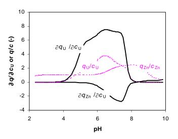
Figure 2. Distribution coefficients  $(q_i/c_i, \text{ dotted lines})$  and flushing factors  $((\partial q_i / \partial c_U)_{i \neq U}, \text{ full lines})$  for Zn and U(6) in acid mine drainage as function of pH.
