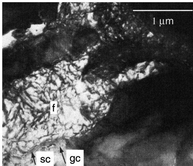
**Fig. 1** Transmission electron micrograph of froth phase (*f*) in a crystalline quartz grain for class 3 Coconino sandstone (sample #33) as modified from Kieffer et al. (1976); *sc* sharp contact, *gc* gradational contact
