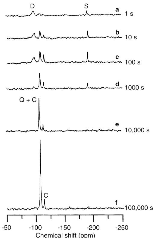
**Fig. 2**  $^{29}\text{Si}$  MAS NMR spectra of Meteor Crater, Arizona sample #33 acquired with a saturation recovery pulse sequence, delay times shown, and MAS=4 kHz. Resonance assignments are for quartz (Q), coesite (C), stishovite (S), and D-phase (D). An arbitrary vertical scale is used for each spectrum in order to emphasize the particular resonances
