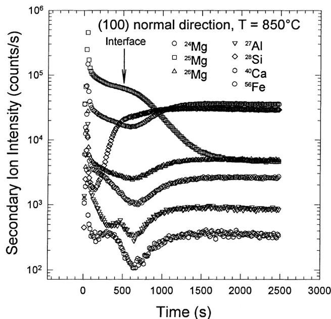
Fig. 2 A typical ion microprobe depth profile analysis with secondary ion intensities plotted versus the analysis time
