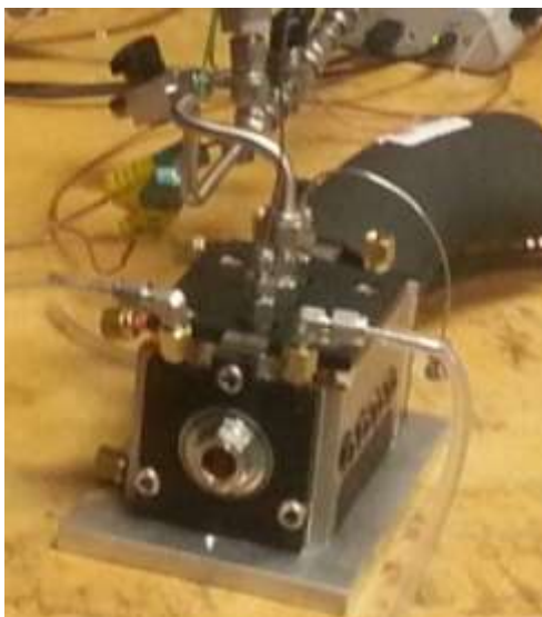
Figure 5-1. Raman spectroscopic cell with sapphire window facing outward. Cell is approximately 10 cm wide.
