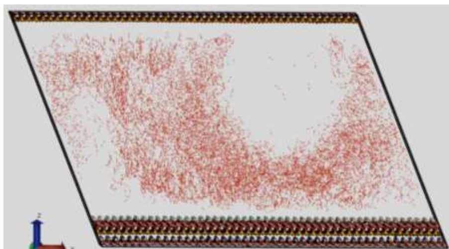
Figure 3-9. A final snapshot taken from a kaolinite nanopore MD simulation at T = 245\text{ K} and P = 1000\text{ bar} . Hydrogen bonding of water molecules is indicated (red) in the montmorillonite nanopore. Hydrate cages can be seen in the lower right corner of the nanopore. Methane molecules have been removed for clarity.
