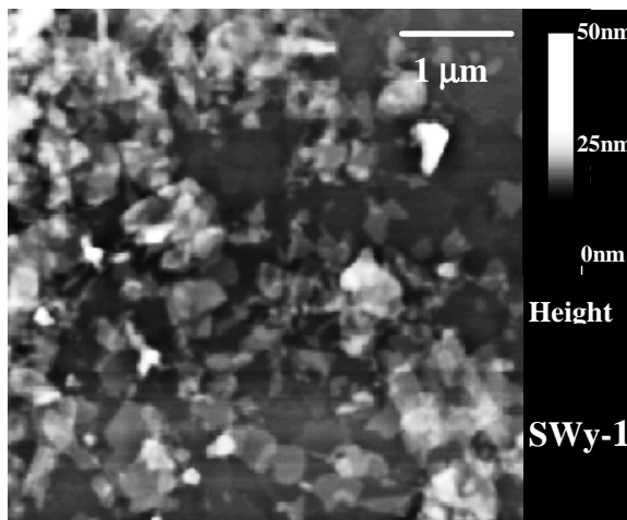
Figure 14. Tapping mode AFM image of Swy-1 montmorillonite; particle size ranges from 0.1-1 \mu\text{m} .
