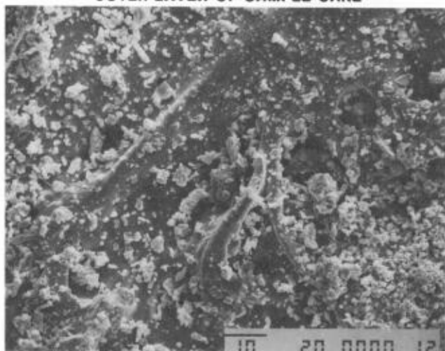
Fig. 5. SEM photomicrograph of oligoclase shocked to 22 GPa, showing morphology indicative of glass formation.
